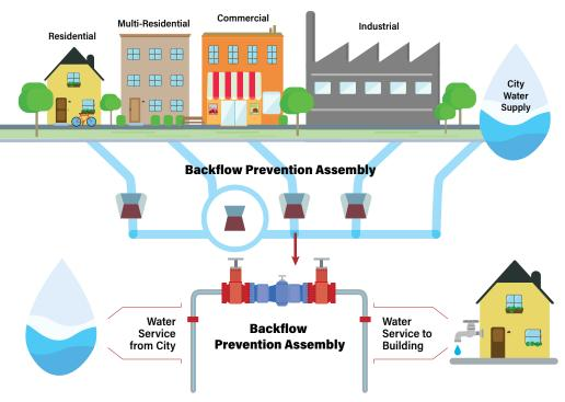
**BACKFLOW:** The undesirable reversal of flow of water or mixtures of water and other liquids, gases, or other substances into the City's water system.
