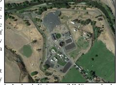
treatment utilizing the modified Ludzack-Ettinger (MLE) method, membranes from the water treatment plant, a membrane bioreactor, a biofuels generator, a sludge dewatering press, and de-chlorination facilities.
