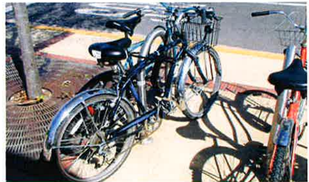
Upside down U or staple rack accommodates two bicycles
