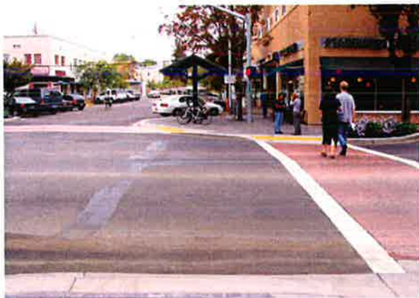
Curb extension provides room for bike parking
