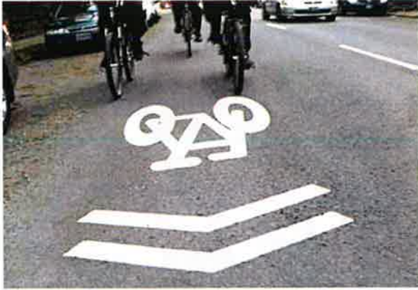
Sharrows indicate where bicyclists should position themselves in the roadway
