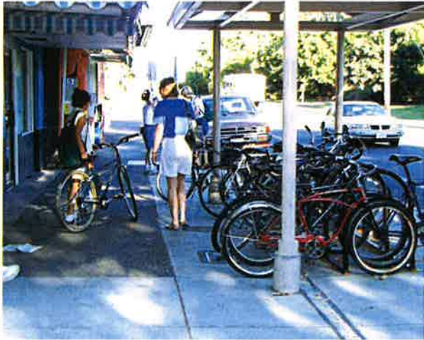
Covered bike parking on curb extension
