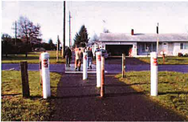
Bollards are overused and can cause injury
