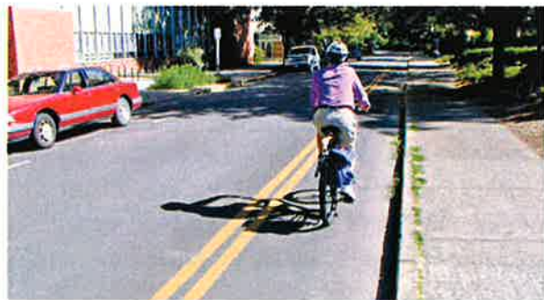
Contra-flow bike lane: One way for cars, two way for bicycles
