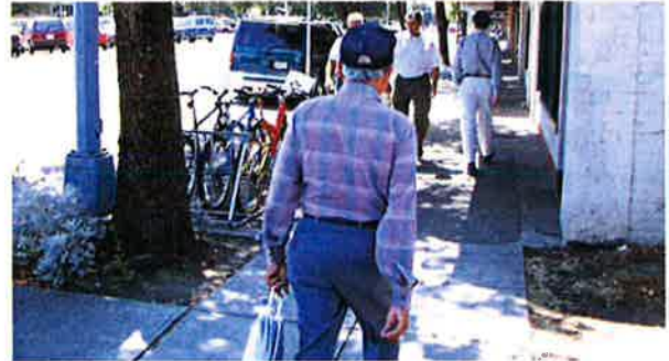
Bike racks placed out of pedestrian zone
