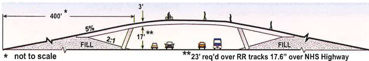
Figure 5-28: Pedestrian overcrossing adds a lot of travel distance when raised above a roadway
