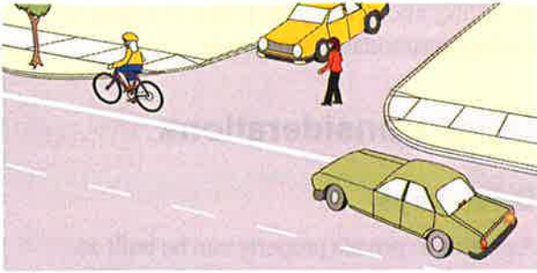
Figure 4-38: Intersection style driveway
