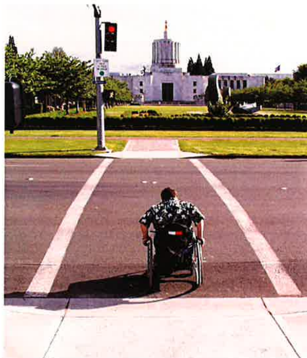
LPI: Pedestrian phase precedes motor vehicle green phase by a few seconds
