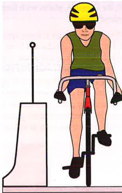
Figure 7-8: Railing added to concrete barrier
