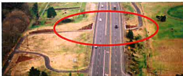
Path is fully separated with an undercrossing
