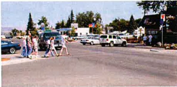
Motorist yields to pedestrians at curb extension
