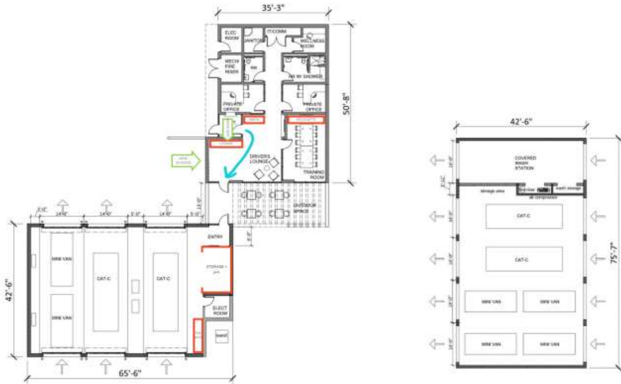
Figure 14 Alternative 1 Bus Barn, Bus Shelter and Administration Building Plans with Workshop Notes
