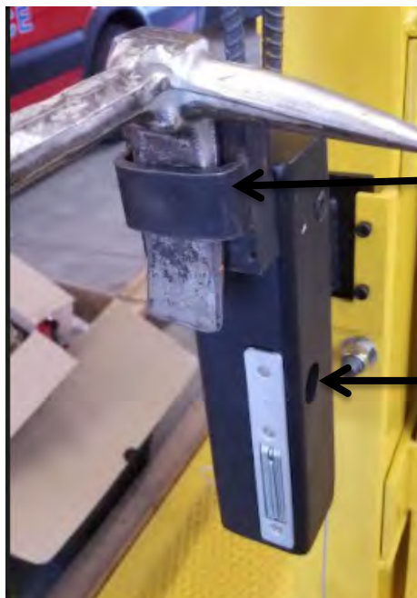
Using the K-tool on the thru the lock cylinder prop. Notice the opening below the K tool on the right for use of the lock pick tools to train on manipulation of a mortise lock swinging deadbolt.
