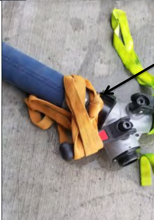
If a gated wye only has one hose operation off of it, the unused valve should be tied shut with a hose strap and clove hitch.
