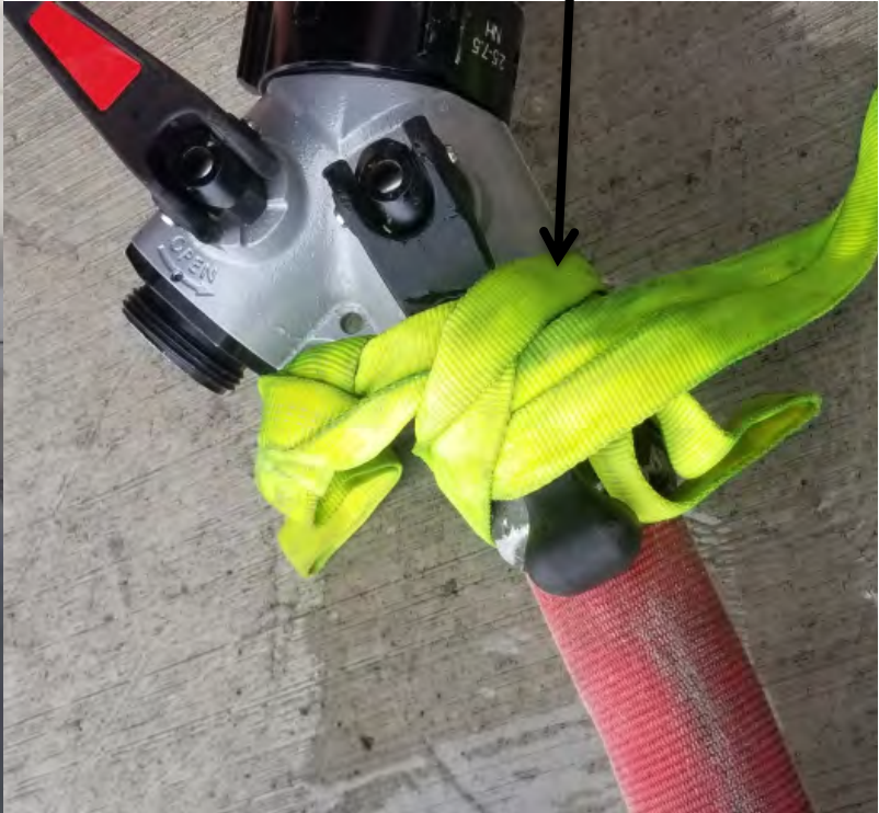
If a gated wye only has one hose operation off of it, the unused valve should be tied shut with a hose strap and clove hitch.
