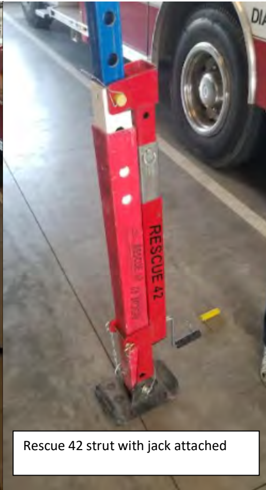
Rescue 42 strut extended with pins placed
