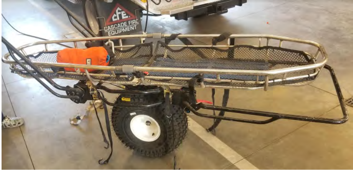
Stokes Basket- A litter widely used in search and rescue. Its key feature is that it can be disassembled for transport.
