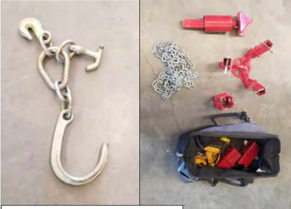
Attachments and accessories shown for the Rescue 42 strut/jacks start on top and moving clockwise: Hook assembly, tripod attachments with base chain, heavy chain for lifting/spreading, and ratchet straps for securing the base to an object.
